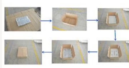
Safety Packaging: PE bag/ bubble bag + foam card + inner box + outer carton
